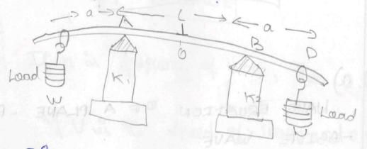
Unitial reading in the miscoscape on the Vortical scale is noted. Equal weights the reading in the miscoscape and Vorticle scale is hoted
