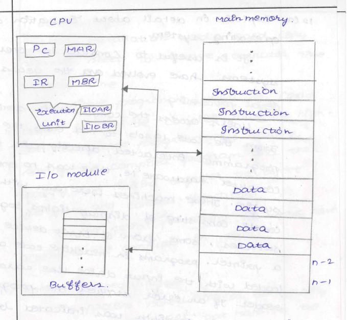
An IIO Buffer Regleter (IIOBR) es used for the exchange of dota between on IIO module and the processor.
