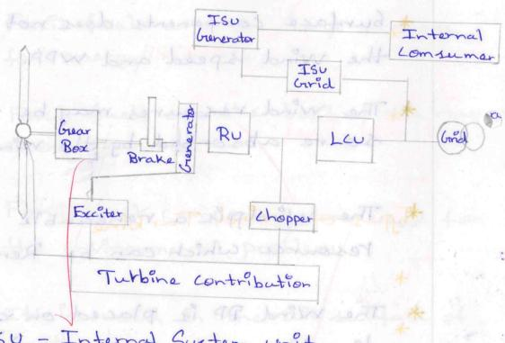
ISU - Internal System unit RU - Rectifier unit
