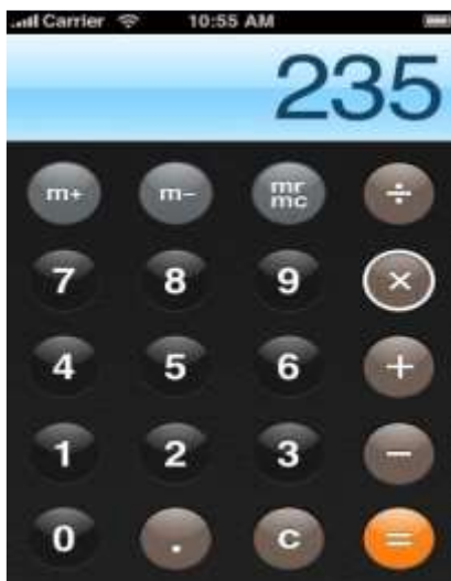
Figure 8-22. The iPhone calculator application uses common fingertip-size controls
