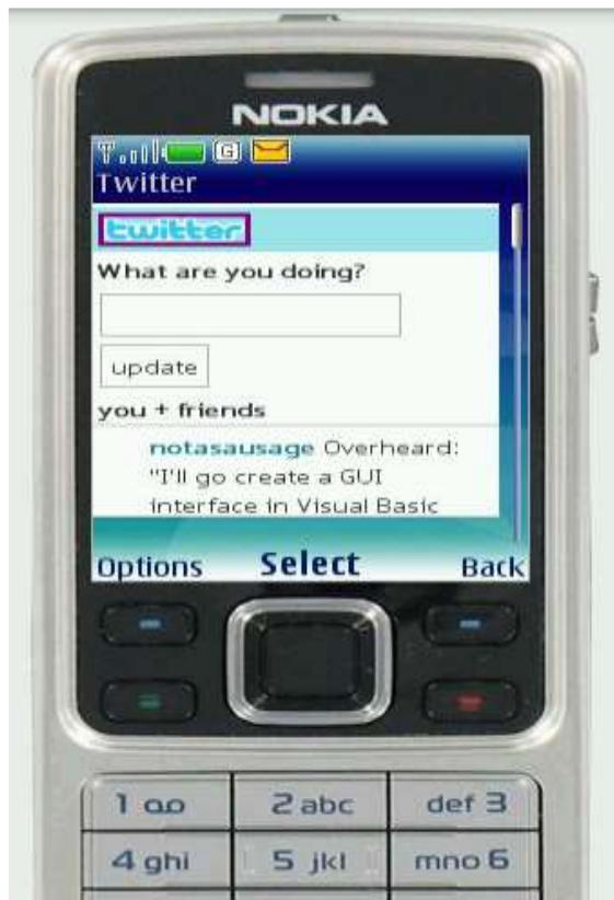
Figure 8-9. Example layout of a scroll-based application, where the user had to press the D-pad past each link to scroll the page
