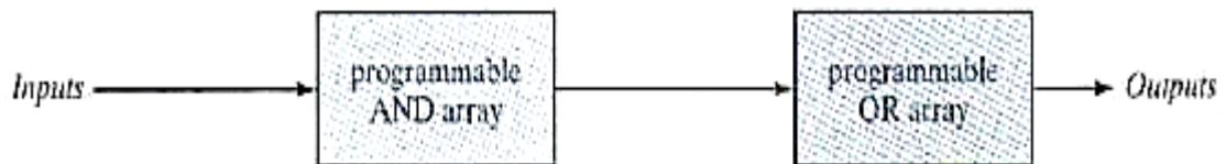
(c) Programmable logic array (PLA)
