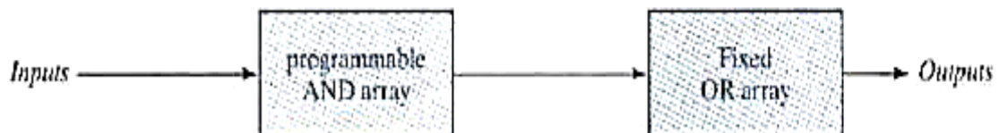
(b) Programmable array logic (PAL)
